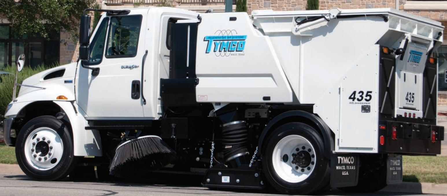
*The Model 435 delivers street sweeping performance in a mid-sized package. With the Conventional Truck Package, the Model 435 has a payload of over 8000 lbs. and overall sweeping path of 132 inches.*
