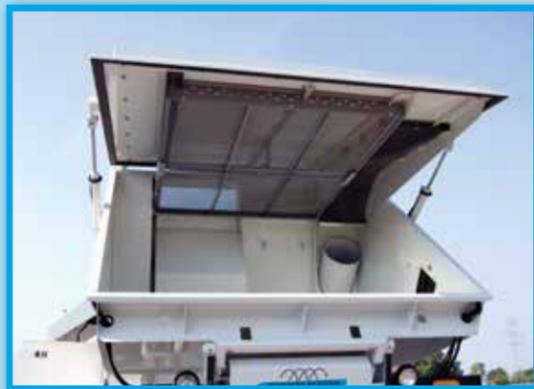
Extra large door allows for easy dumping and cleaning.
