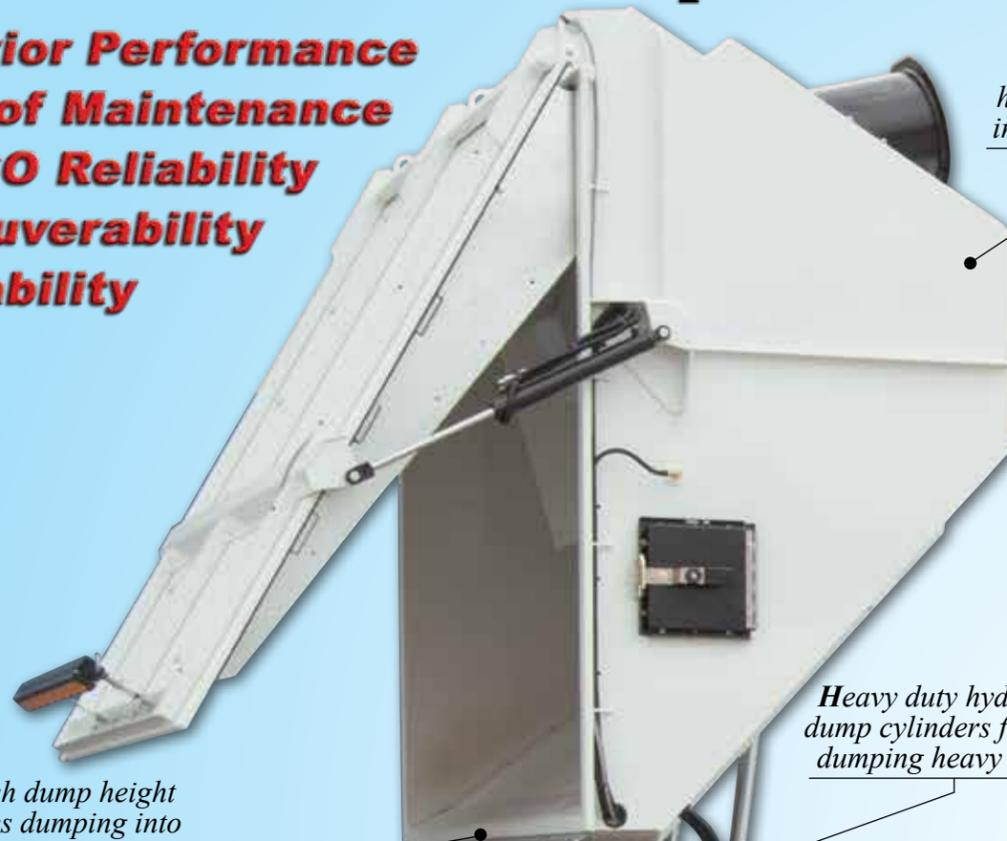
Large 4.0 cubic yard heavy duty, steel hopper increases sweeping time.
